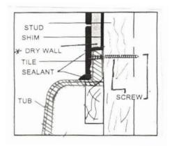
\* Drywall or cement board may go over tile flange and rest on top of tub or stop at top of tile flange. The tile must go over tub lip and rest on top of the tub.
